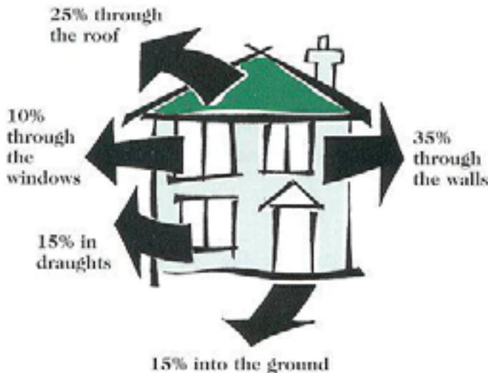
As illustrated in the diagram, the majority of heat loss in a typical dwelling is through the walls, windows and roof. Medium density housing is a viable and efficient housing choice because shared walls and ceilings help to retain heat within the building.
