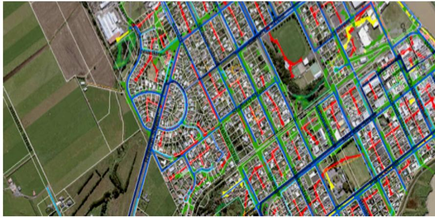
With a number of options available to us (including on site soakage, on site tanks and reuse, pond detention, rain gardens etc.), there will be no change increase in the maximum stormwater flow for a given design storm. This is normally designed for the 1 in 100 year storm.
