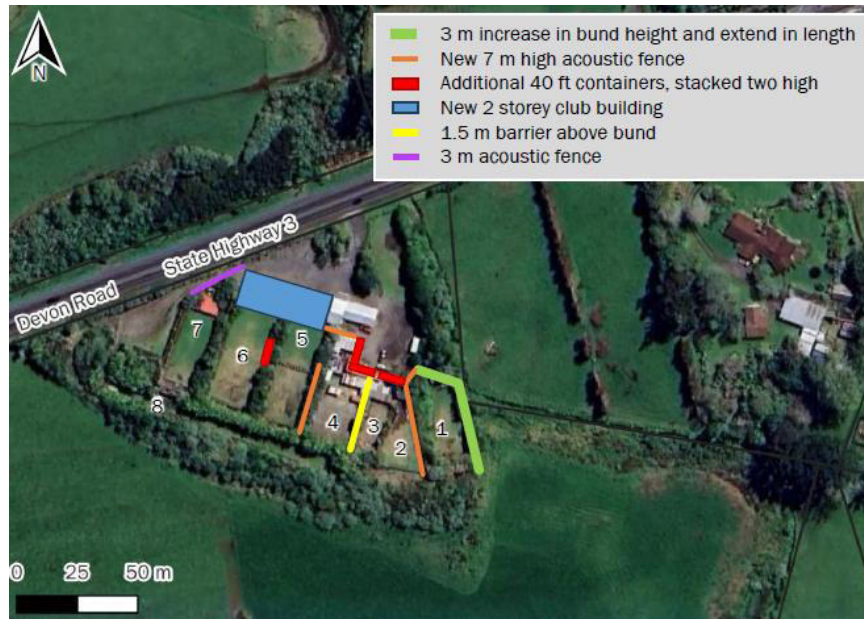
Figure 3.1: Recommended physical noise mitigation measures (source: AES, 2024)
