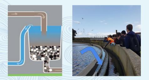
The tiny bugs are separated from the water in the clarifier.
