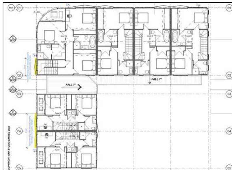
Figure 3: First and Second Floor Encroachment of window screens (highlighted) on the North Building
