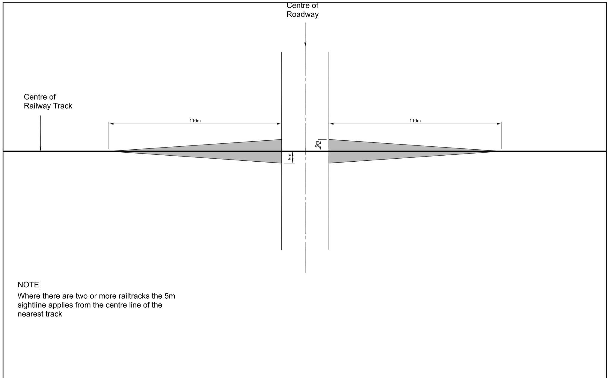
Diagram 19.2 Railway level crossing sightline distances at controlled crossing with 70km/h maximum railway line speed
