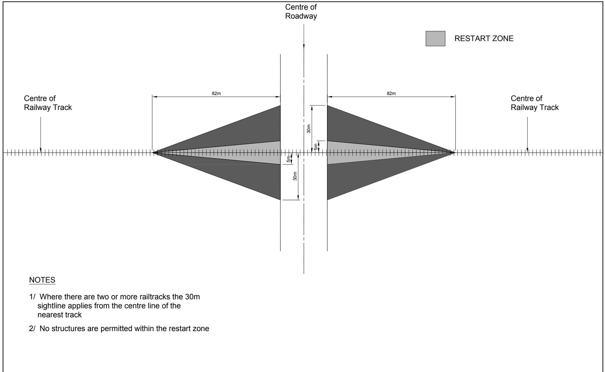
Diagram 19.4 Railway level crossing sightline distances at uncontrolled crossing with 70km/h maximum railway line speed
