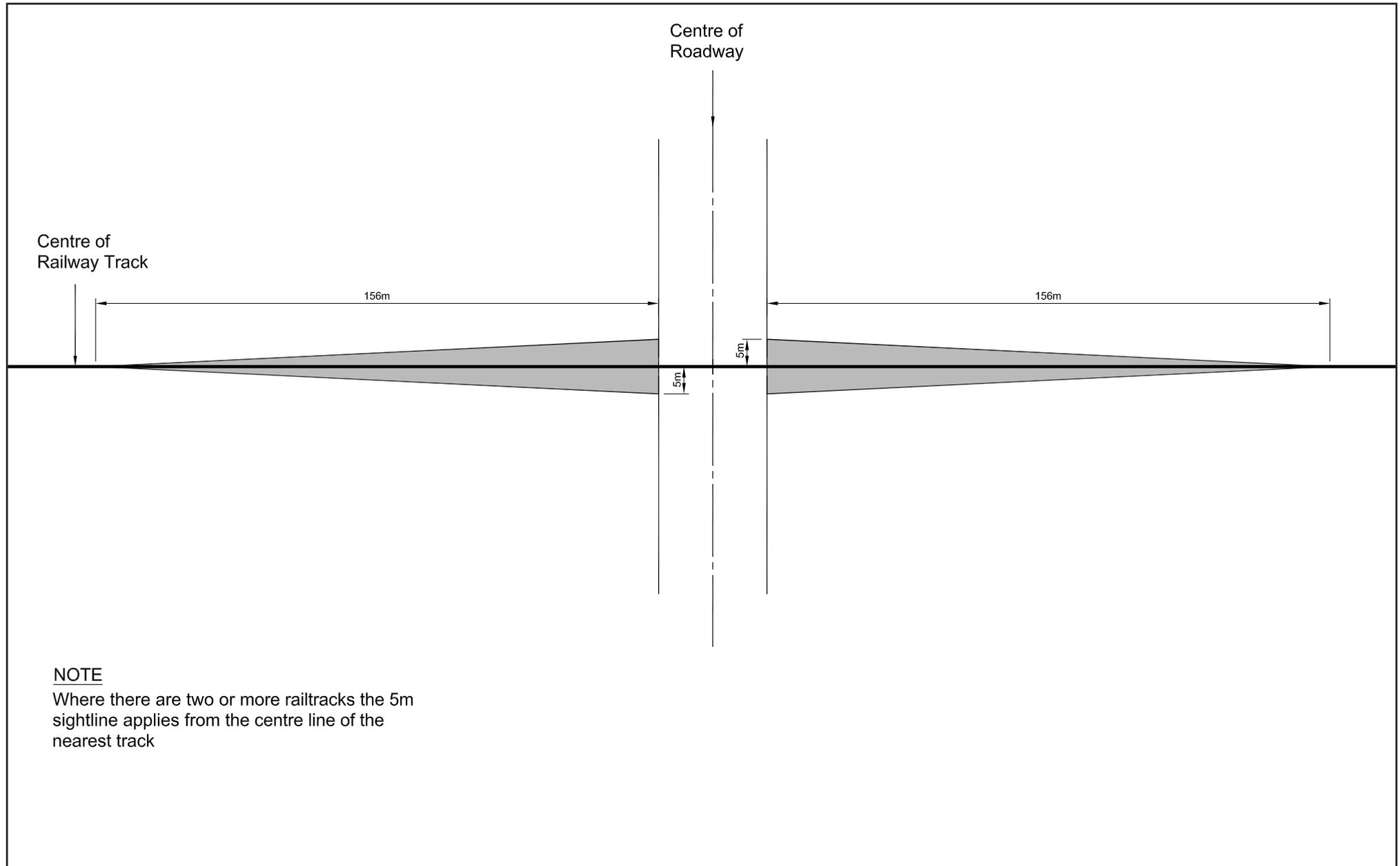
**Diagram 19.3** Railway level crossing sightline distances at uncontrolled crossing with 50km/h maximum railway line speed (refer to diagram 19.5 to identify this area)
