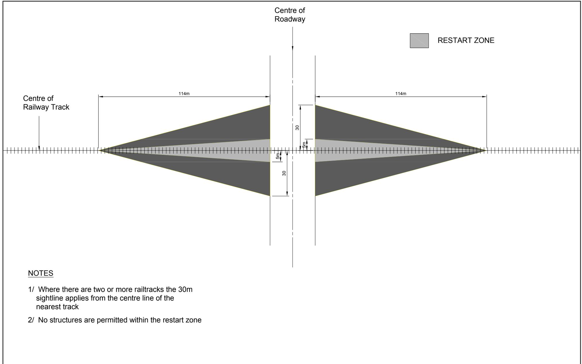
**Diagram 19.5** Location of railway track where maximum line speed is 50km/h
