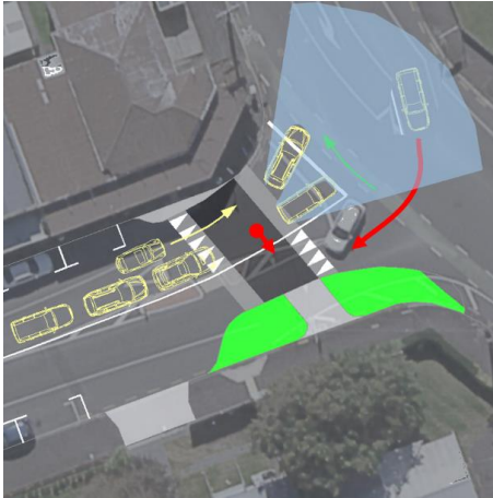
Figure 4. Indication of risks associated with Amended Design of raised safety platform, Huatoki Street.
