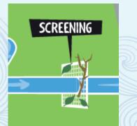
Water is screened after collection. Any leaves or bits of debris are removed from the pipe before it gets to the water treatment plant.
