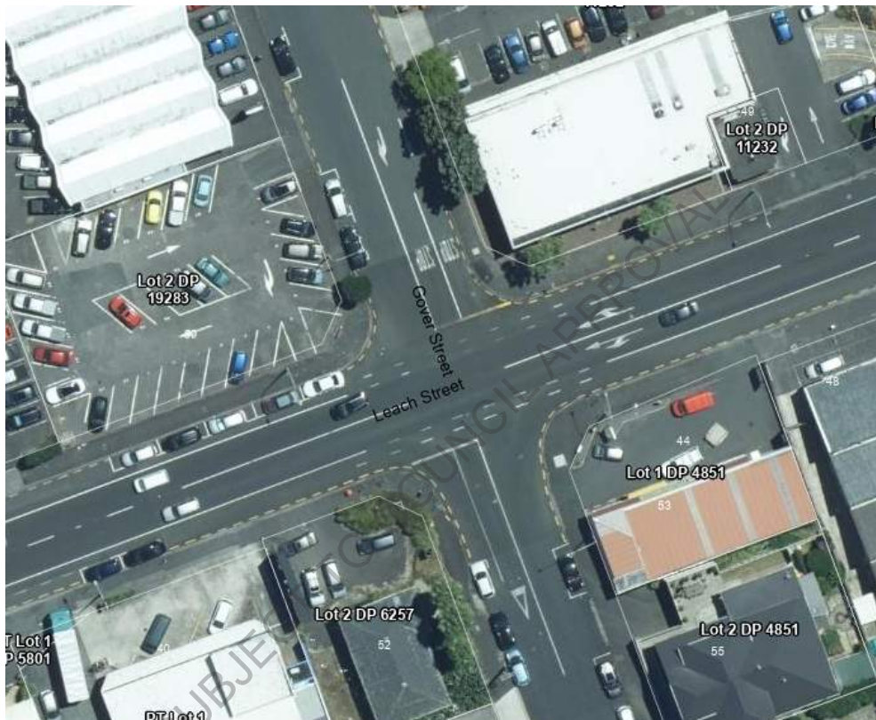
Figure 4-20: SH45 (Leach Street) with no crossing facilities
