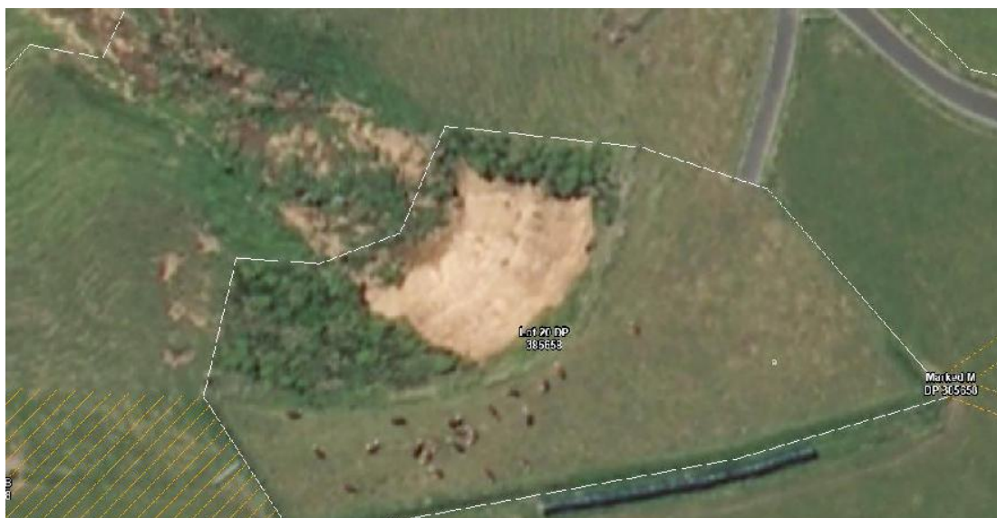
Figure 2.3: Aerial photo showing landslip on the gullyhead slope in 2012 3
