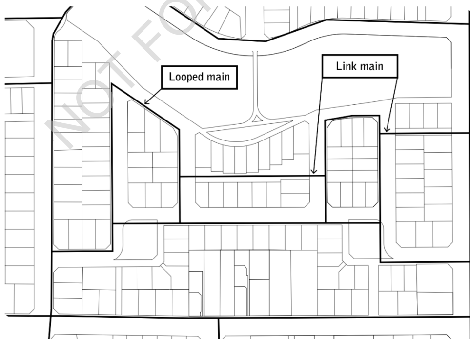
Figure 6.4 - Elimination of termination points
