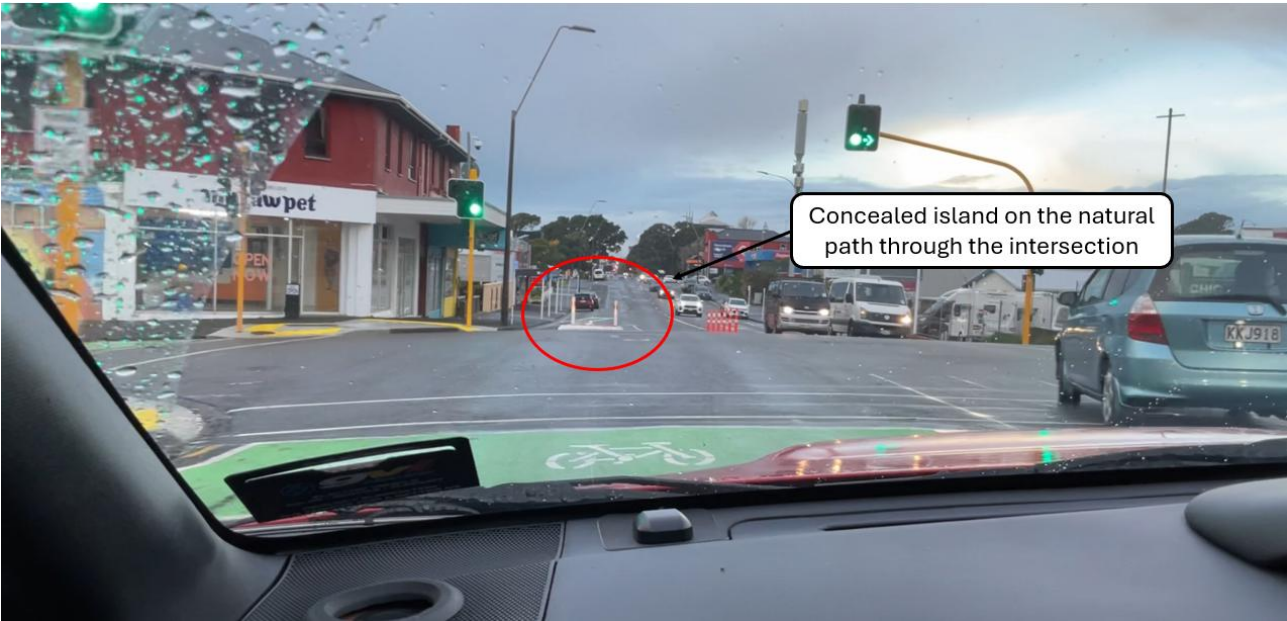
Figure 4-13: Concealed island in the natural path of vehicles heading eastbound through the intersection.
