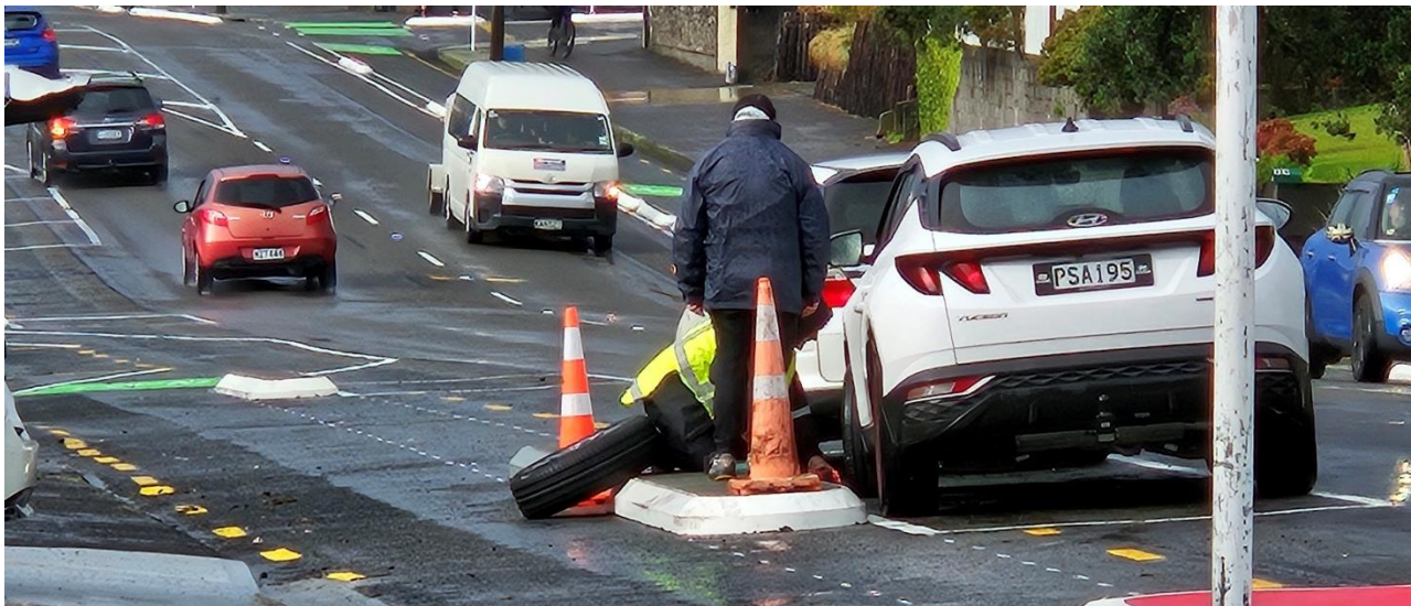
Figure 4-6: Damage vehicle due to collision with the concrete cycleway separator on SH45 / Devon Street West
