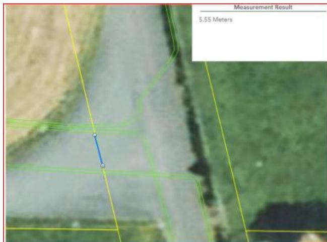
Fig two: Pipeline width within road reserve shown in blue, existing pipelines are shown in green and are discussed further within this report.
