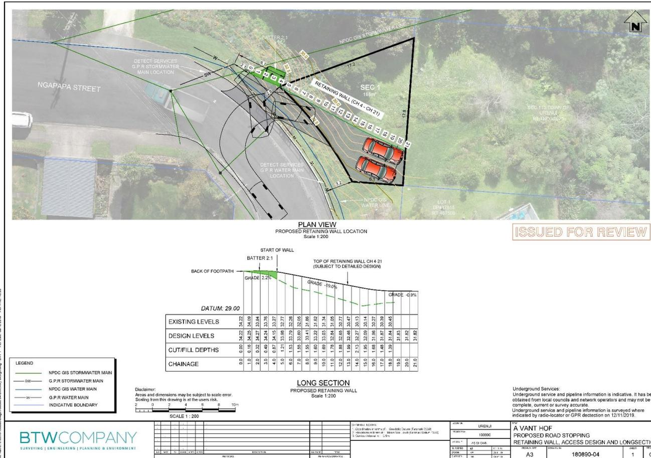
Figure Four – Proposed Retaining Wall, Access design and Longsection
