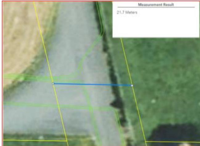
Fig one: Pipeline length within road reserve shown in blue, existing pipelines are shown in green and are discussed within this report.
