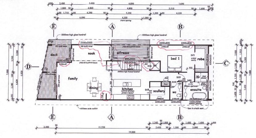
raking studs (exterior stud spacing 600mm crs) 2200mm window head heights Insulation: walls -R2.2, ceiling -R3.2
