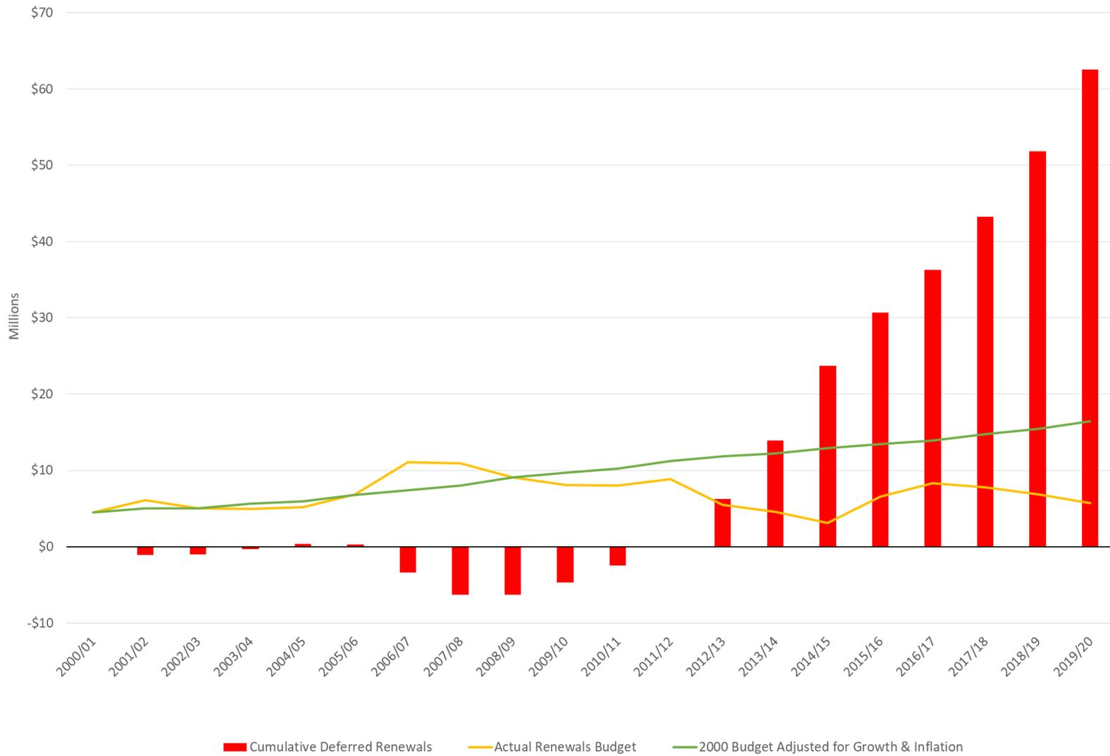
Figure 5 – Capital Budgets compared to the 2000 budget adjusted for growth and inflation as well as the cumulative value of deferred renewals.
