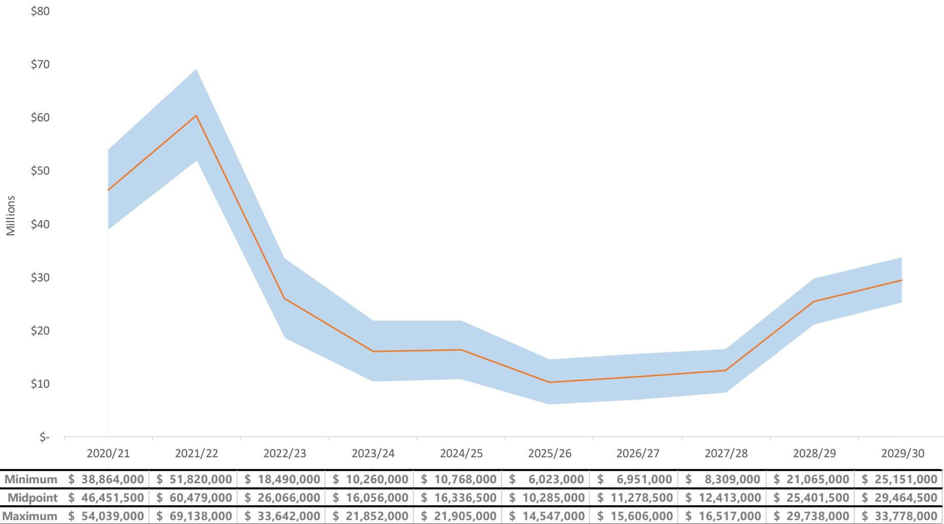
Figure 13 – 10 Year Renewal Forecast bringing together Remaining Useful Lives, Condition and Criticality where reliable data is available.
