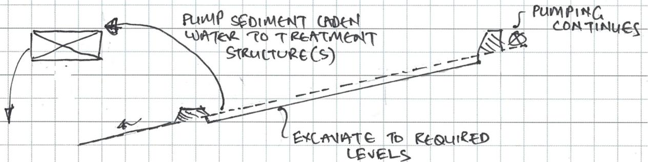
**STAGE 3: LAY PIPE (USING METHOD A OR B), INSTALL INTAKE & OUTLET STRUCTURES, AND FILL TO FORM SRP PLATFORM**
