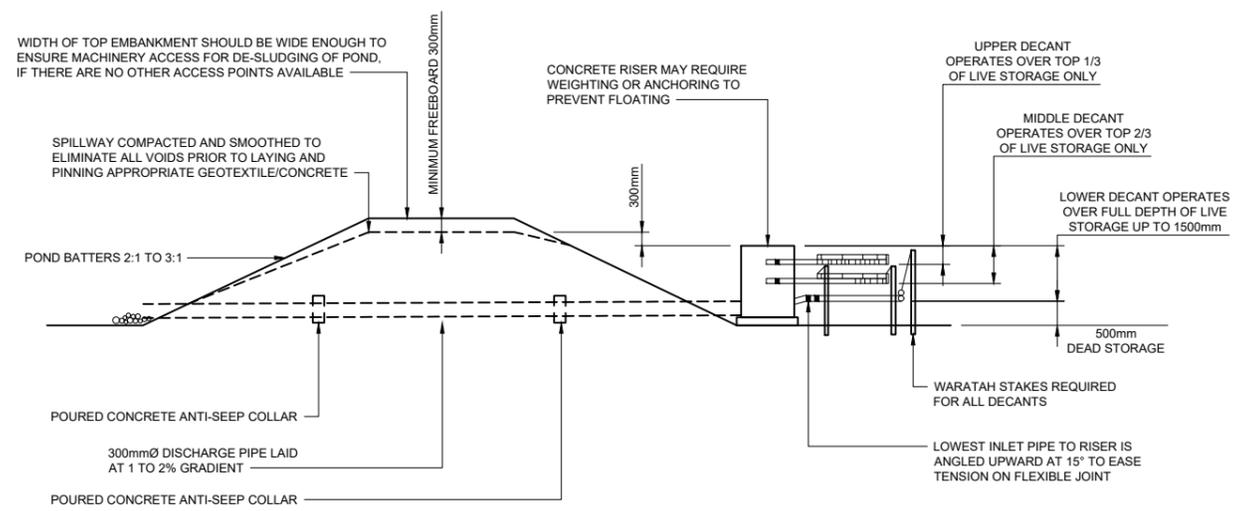
SECTION - SEDIMENT RETENTION POND FOR THREE DECANTS
