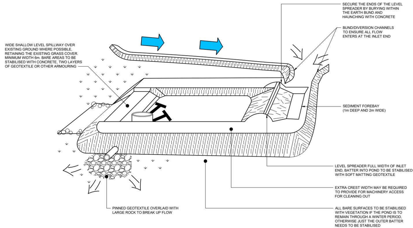
SCHEMATIC - SEDIMENT RETENTION POND
