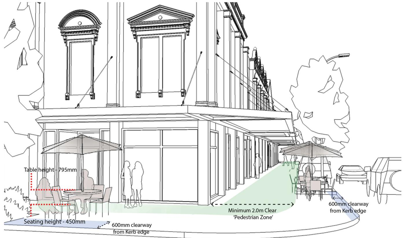
**Figure 5:** Diagram showing minimum 2.0m pedestrian zone, and preferred table heights and setbacks from street edge.
