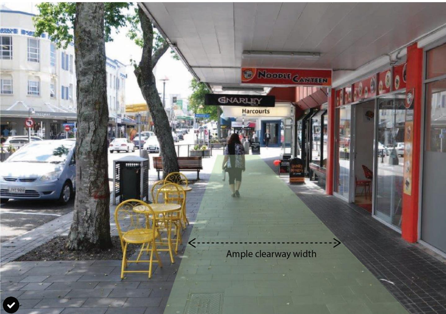
**Figure 6:** Existing Devon Street (southern side of street) showing clear pedestrian zone width, minimum 2.0m.
