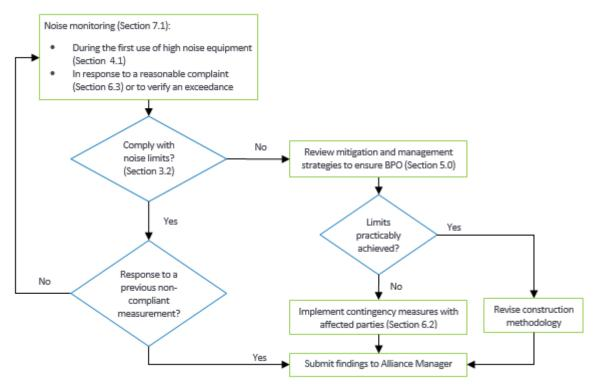
Figure 7.1 - Noise Monitoring Flow Chart
