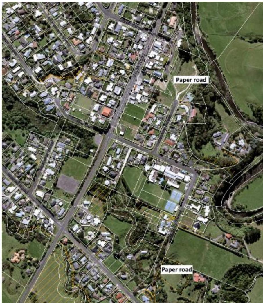
Donnolly St has a sealed width of 8m from the state highway to the school where it widens to 13.2m and turns through 90° and narrows to 5.7m.
