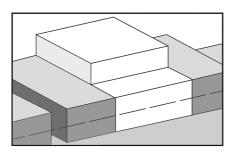
Reducing height close to the street edge and using upper level setbacks moderates the height difference between new and existing buildings.
