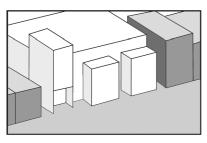
Placing smaller foreground elements along the street frontage helps to reduce the impact of bulk and aids the scale relationship to adjacent buildings
